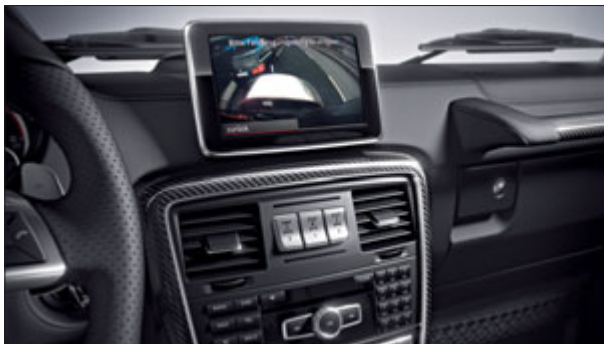
During parking, the COMAND Online central display shows the area behind the car.
