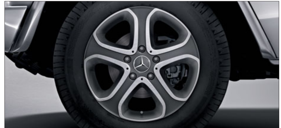
5-spoke light-alloy wheels with 265/60 R 18 tyres, painted titanium grey with high-sheen finish (standard for "Final Edition 200" and Sports package, optional for G 350 BlueTEC, G 500, Code RL5).
