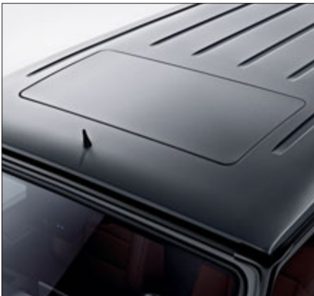
Sliding sunroof, electrically operated (for Station Wagon).
