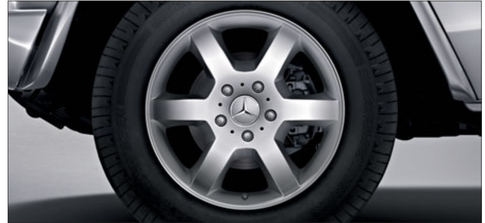
6-spoke light-alloy wheels with 265/60 R 18 tyres, with high-sheen finish (option for G 350 BlueTEC, G 500, Code RL6).
