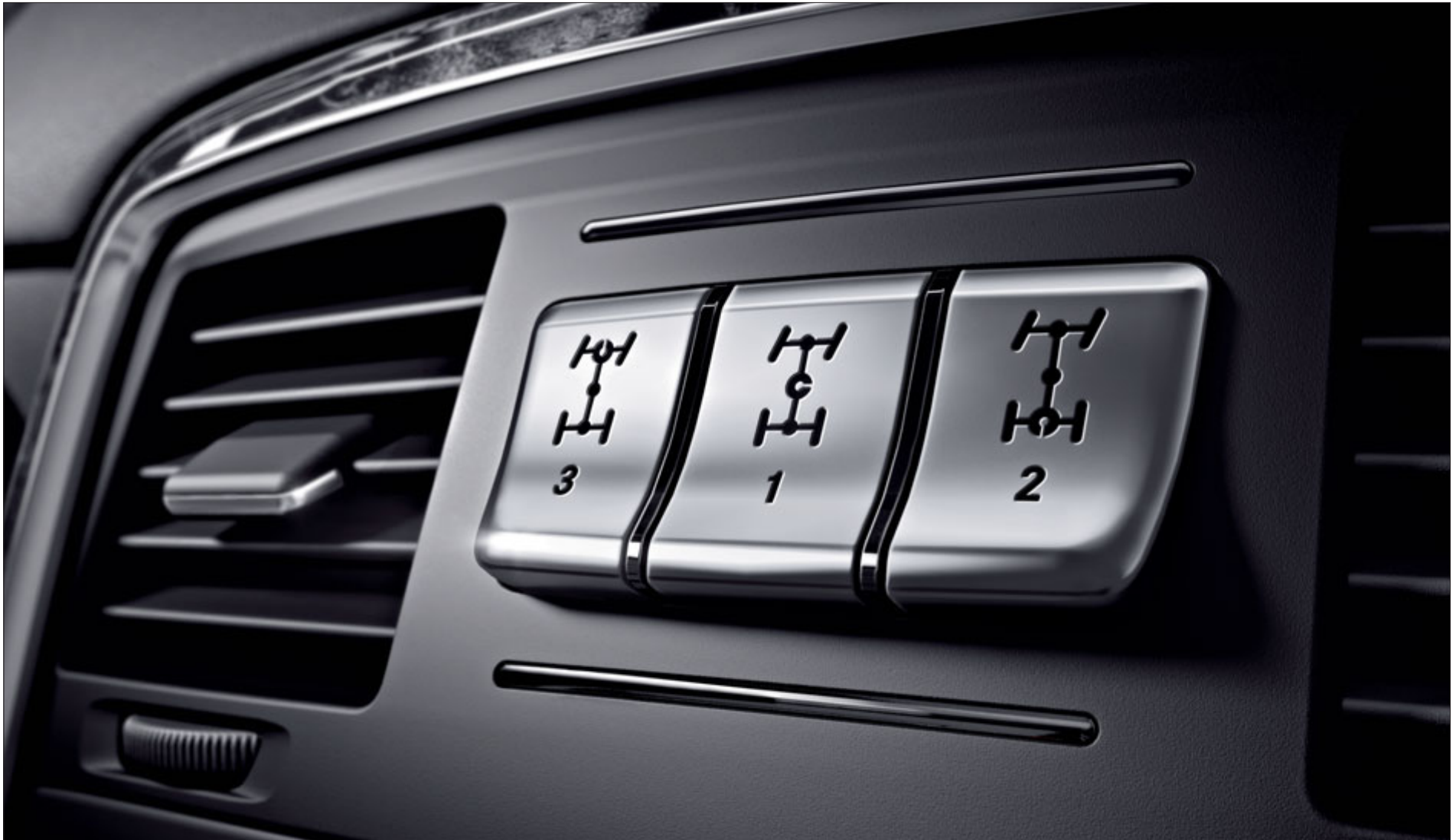
The three electrically engageable fully lockable differential locks play a key role in the off-road capability of the G-Class.
