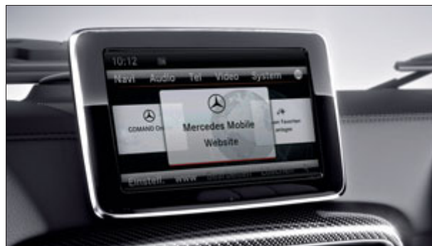
The multimedia system with HDD navigation has a high-resolution display with TFT technology with a 17.8 cm screen diagonal.
