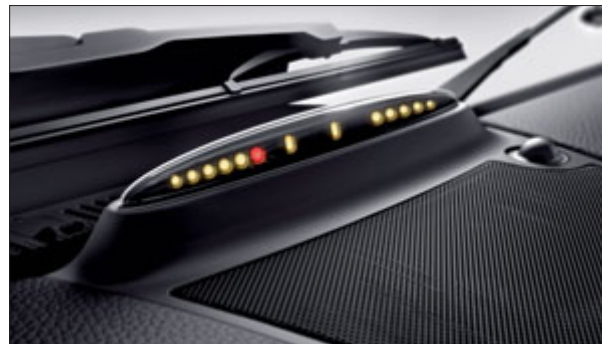
The light-emitting diodes of the PARKTRONIC system indicate the distance to an obstacle.
