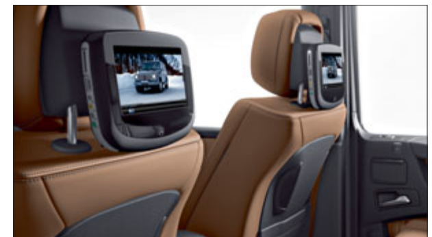
The two displays of the Rear Seat Entertainment System mounted on the front-seat head restraints.
